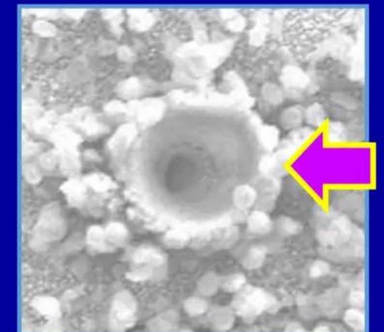
100 \mu LENR crater in Pd cathode LENR electrochemical cell
