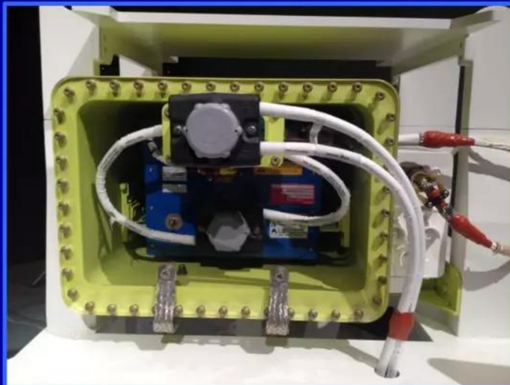
New battery case installed inside stainless steel containment box
