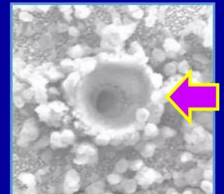
100 μ LENR crater in Palladium Electrochemical LENR cell
