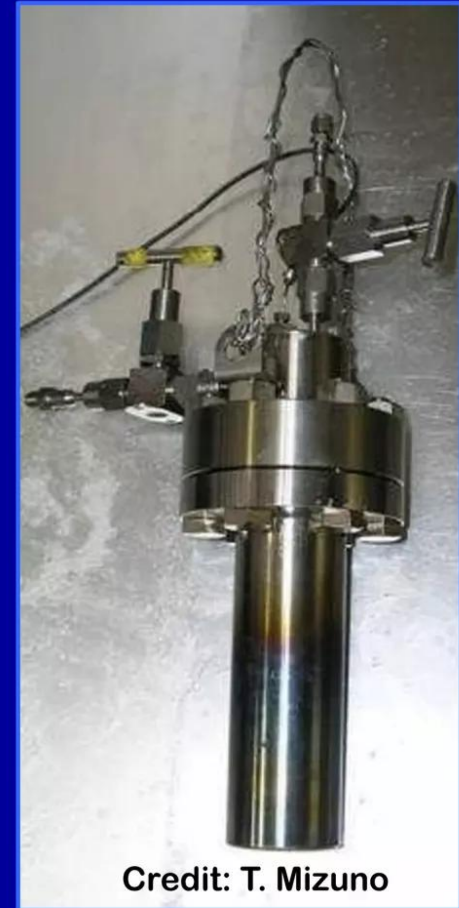
Hydrogen gas-filled Inconel 625 stainless steel reactor vessel
