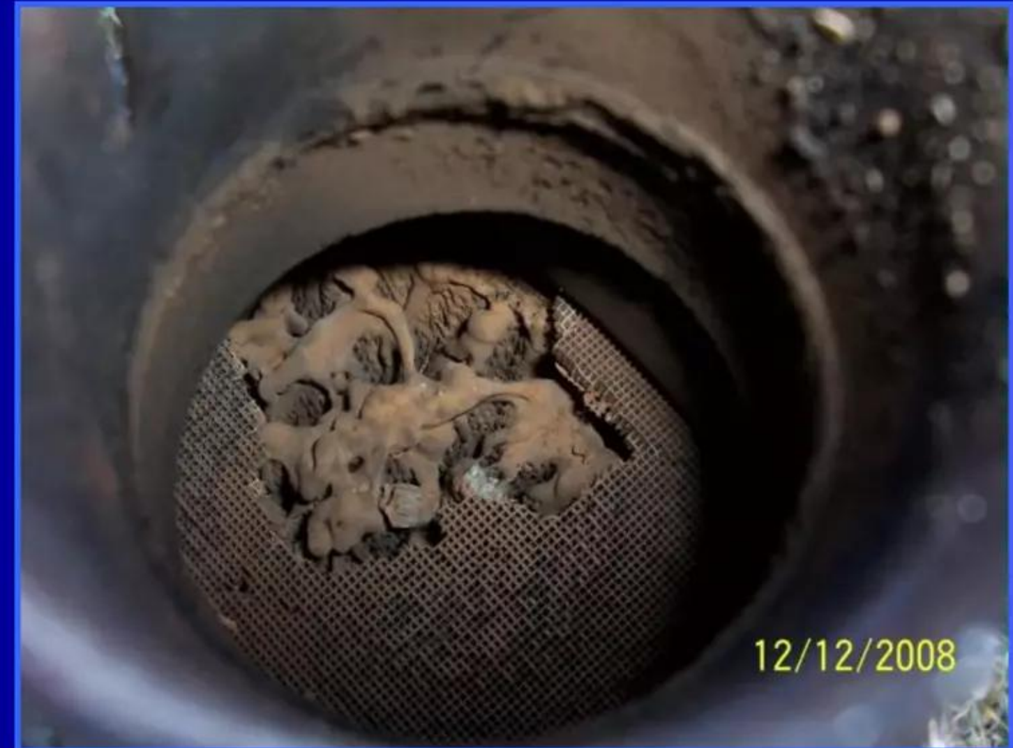
Top: broken piece of ceramic honeycomb Bottom: melted honeycomb post thermal runaway
