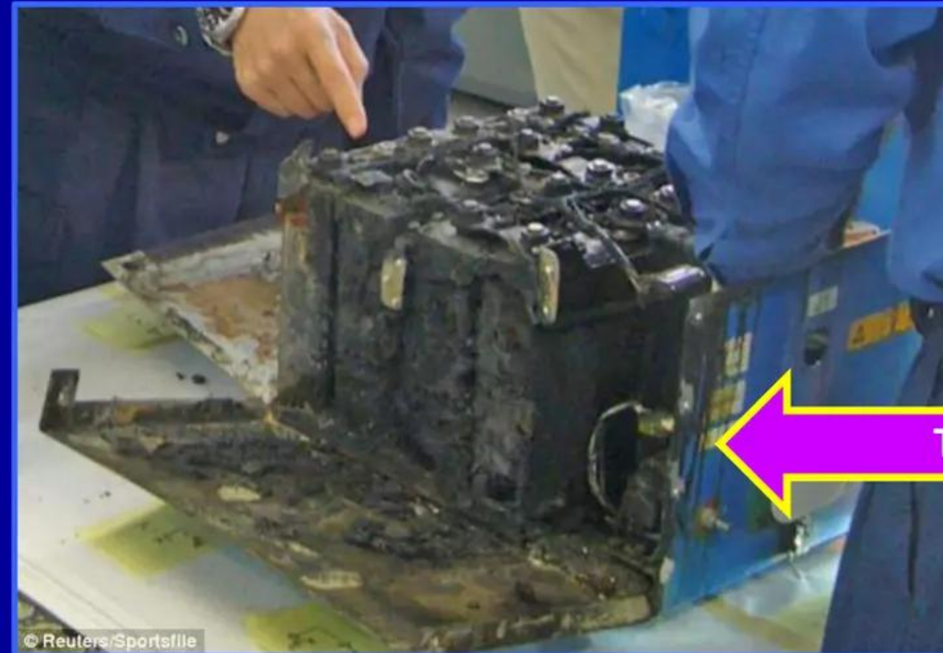
Severely fire-damaged GS-Yuasa Li-ion battery pack involved in Logan Airport 787 incident (NTSB)
