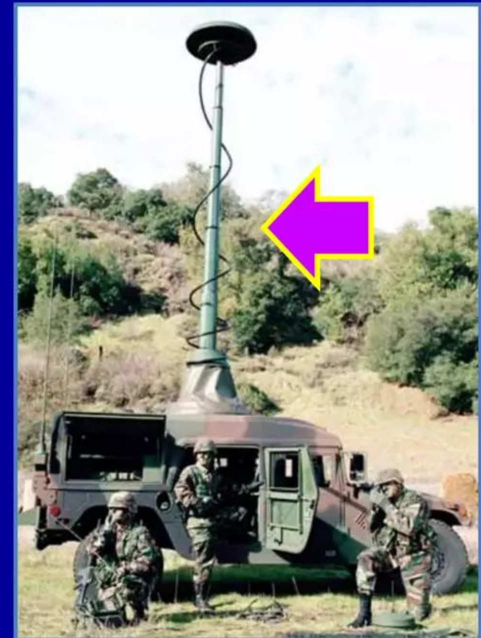
Cobham EXB or EXL carbon-fiber telescopic masts- can be hand cranked
