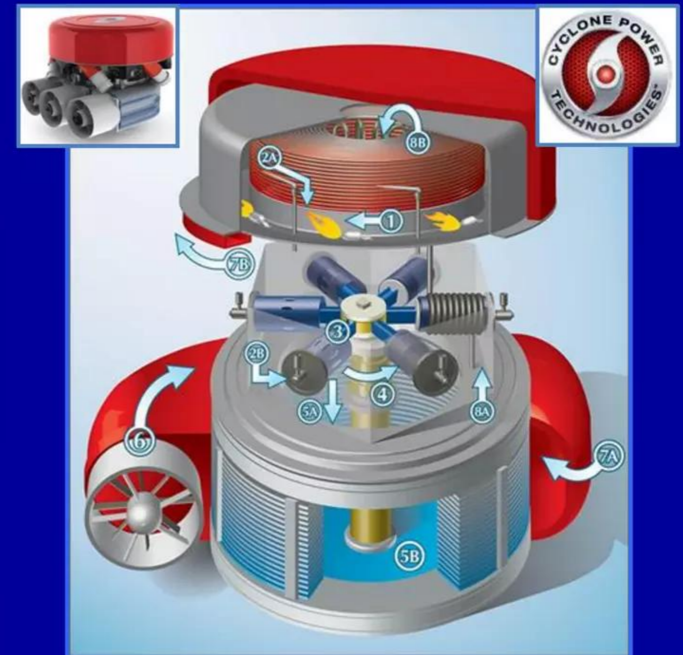
Modified Rankine cycle steam engine by Cyclone Power Technologies
