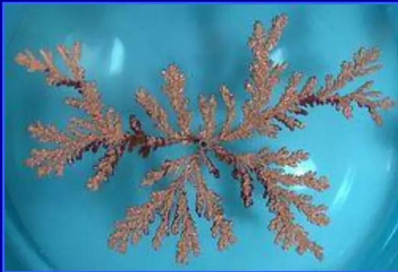
Image: macroscopic cm length-scale Copper dendrite growing in aqueous Copper Sulfate solution
