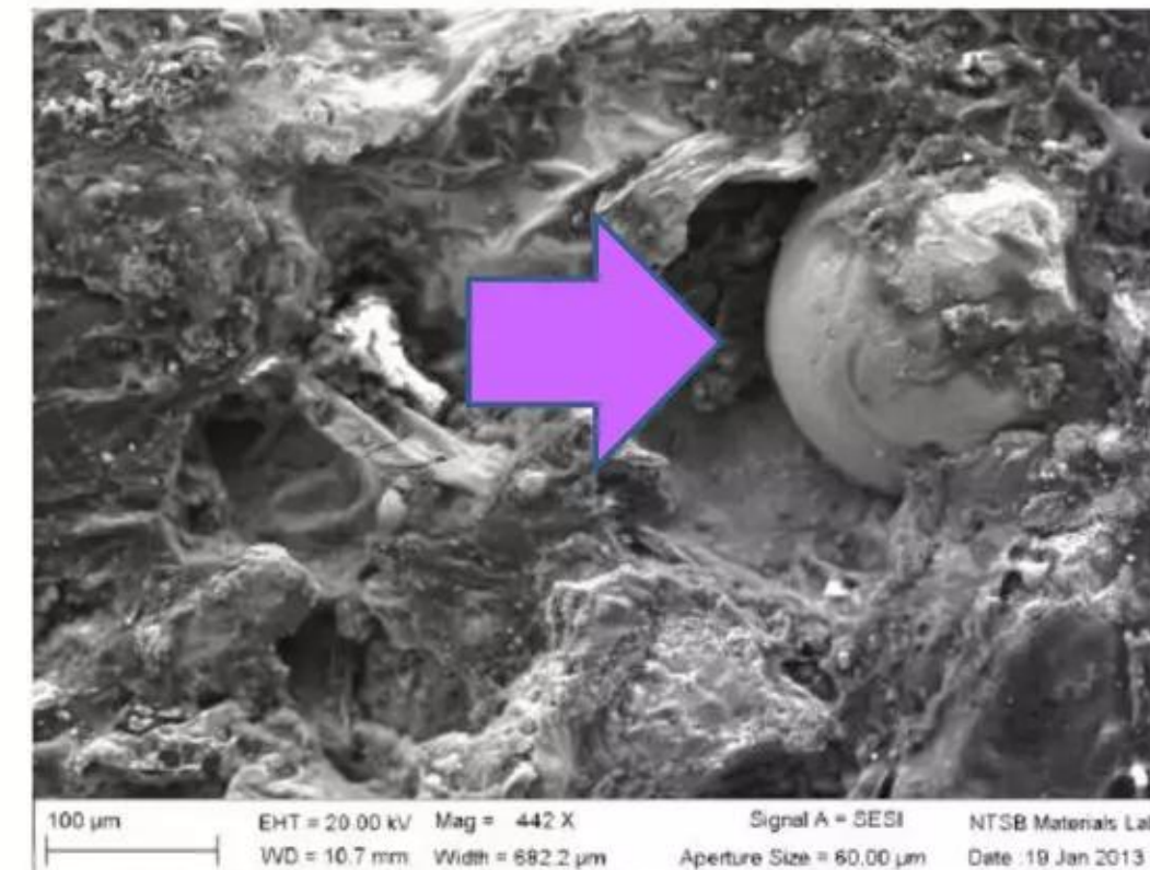
Figure 66. SEM micrograph of steel sphere embedded in combustion products in the interior of hole 1 on the C5 cell case.
