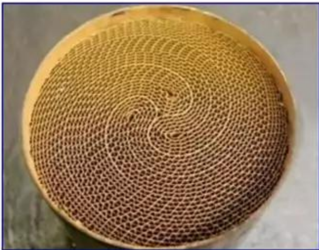
End view: metal honeycomb
