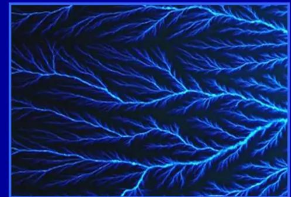
Image: mm length-scale Lichtenberg Figures from electrical discharge through plastic
