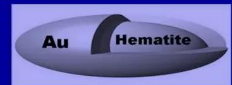
High local SPP electric fields surrounding "nanorice" - Au coating on hematite core
