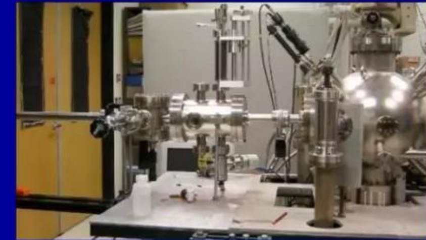
Pulsed Laser Atom Probe Microscope at NWU, Source: :Fig. 7, pp. #9, Seidman & Norem proposal (2005)
