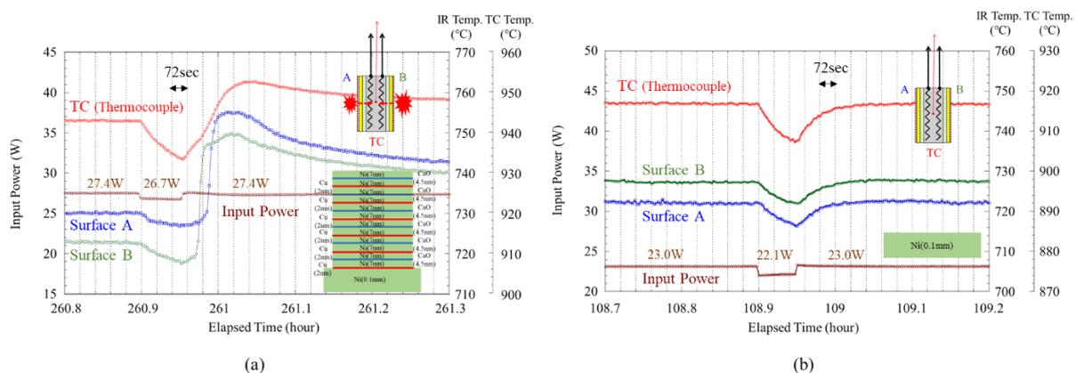
Figure 1. Different responses of sample surface and heater center temperature to input power perturbations: (a) An example of heat burst by an intentional input perturbation, (b) An example of no heat burst by a similar input perturbation.
