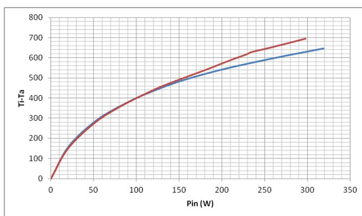
Figure 2. trend of the powder temperature as a function of the input power for one of the tests where the thermal anomaly is more evident. It is observed for the temperature of the powder that around 450 the power to reach the same temperature in the case of the hydrogen test is lower than that of the calibration up to about 60 W at 620 degrees. (the temperature trend for the test with H<sub>2</sub> is in red color)
