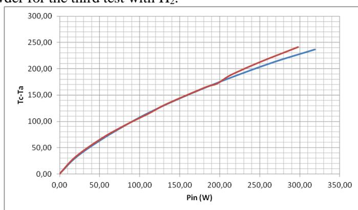
Figure 1. Reactor temperature trend as a function of the input power for one of the tests where the thermal anomaly is more evident. It is observed that around 200 W of input power, a significant deviation of the reactor temperature for the cycle in Hydrogen compared to the reference test in Helium. (the temperature trend for the test with H<sub>2</sub> is in red color)
