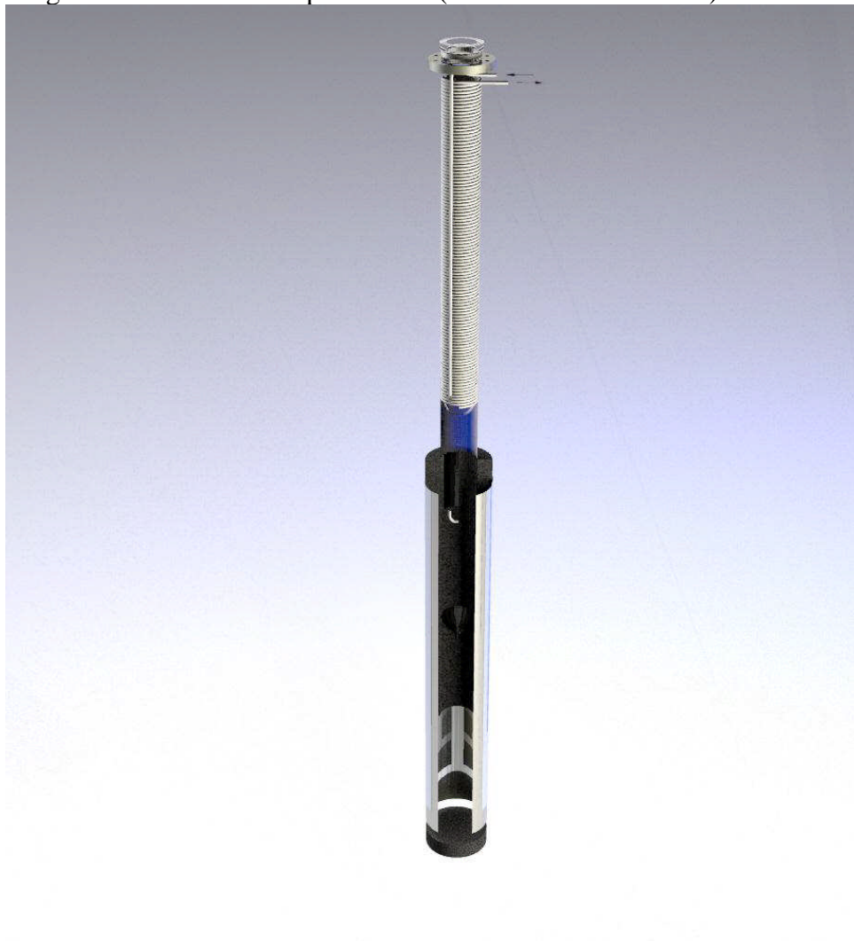
Figure 13. Schematic of assembling procedures of glass reactor, heat exchange system and outer thermal insulation.
