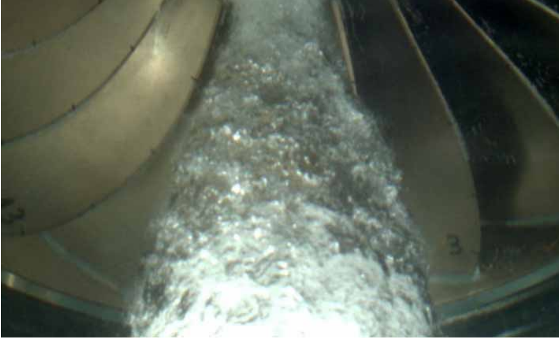
Figure 3. Cavity under runner in Model Test
