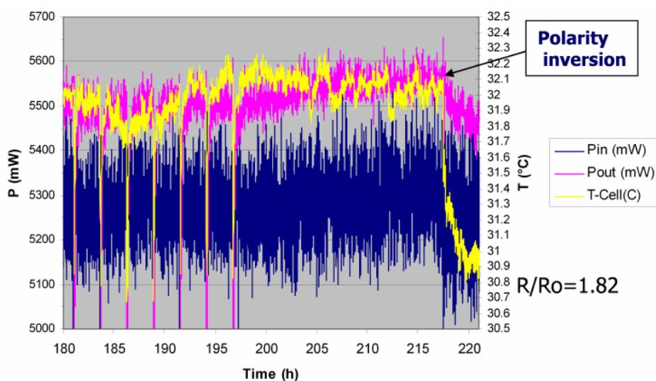
Fig. 8. Temperature and Output Power decreasing after changing electric polarity.  $P_{in}$ =constant
