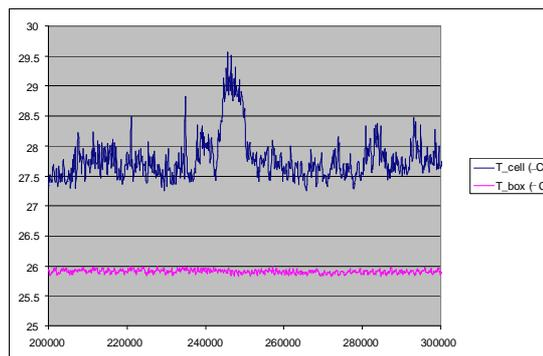
Fig. 7. Electrolyte temperature evolution: the temperature increase is well correlated with excess power.
