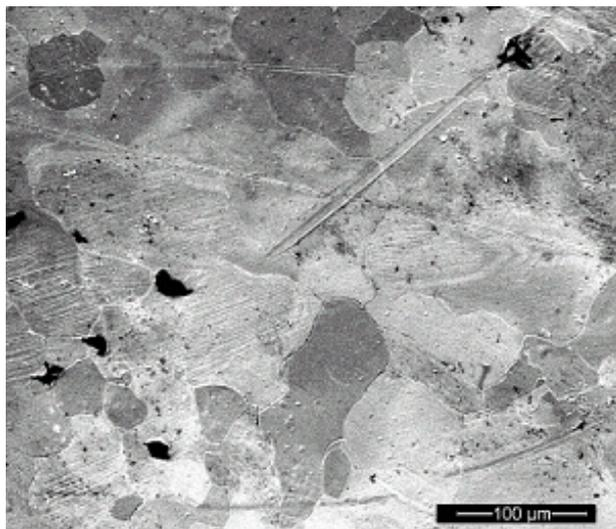
Fig. 1. Pd cold worked and annealed.
