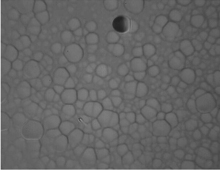
**Figure 16.** Typical image of the front side of #5 detector after total 21 hr etch (real nuclear tracks in the background of the “ground beef”). The bright oval track at lower part of the figure was made by a proton with oblique incidence. The dark circle at the upper part of the figure was made by an  $\alpha$ -particle.
