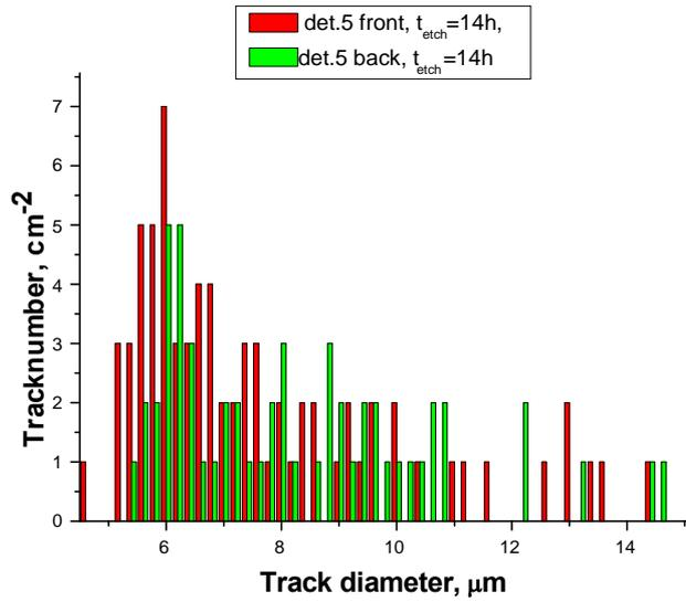
**Figure 18.** Comparison of the front and the back sides of the proton recoil spectra of the #5 detector at  $t = 14$  hr etch.
