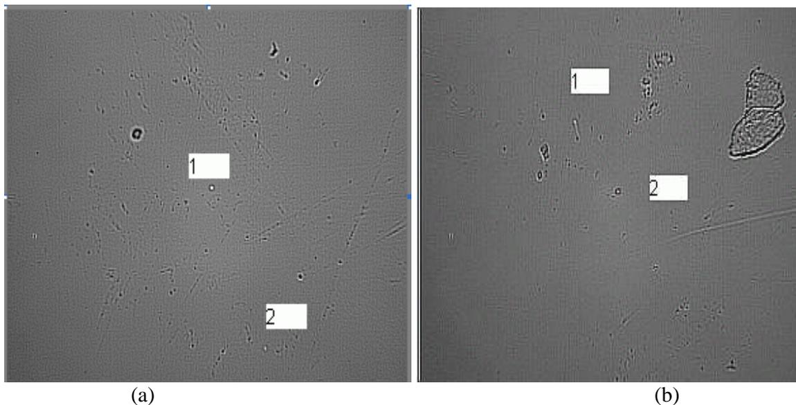
**Figure 5.** Examples of proton recoil tracks (compare with Cf-252 bright pits) of 5-7  $\mu\text{m}$  diameter from CR-39 foreground detector #7 (removed depth is  $h \approx 8.6 \mu\text{m}$ ), images size is  $S = 120 \times 90 \mu\text{m}^2$ : (a) - two tracks of normal incidence (1,2); (b) – track of oblique incidence (1), track of normal incidence (2).
