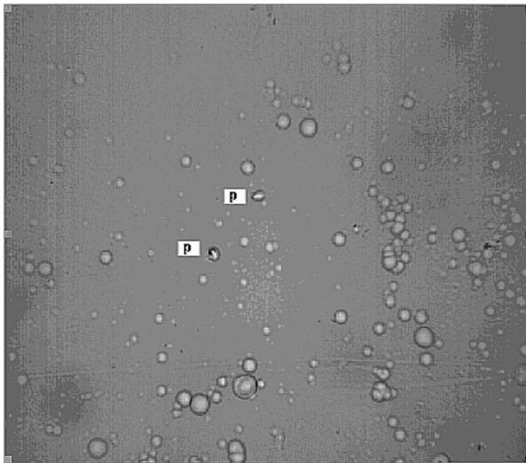
**Figure 15.** Proton recoil tracks at the front side of #5 detector well distinguished among the defects (so-called “ground beef”) background at  $t = 14$  hr etch.
