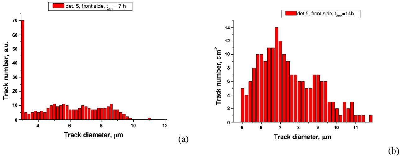
**Figure 14 (a,b)** Individual pit density at the front side of #5 detector: 7 hr (left) and 14 hr (right) etch.
