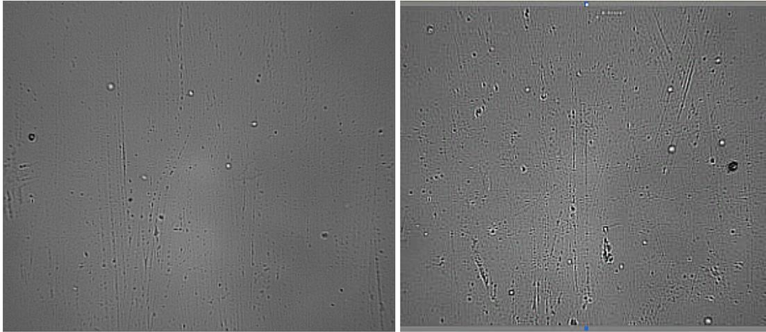
**Figure 4.** Examples of proton recoil tracks of 5-8  $\mu\text{m}$  diameter (bright pits only - all others are surface defects!) for Cf-252 neutron source (7 hr etch, removed depth is  $h = 9.2 \mu\text{m}$ ). Total neutron fluence is  $F_n = 7 \times 10^8 \text{ n/cm}^2$ ; the size of each image is  $S = 120 \times 90 \mu\text{m}^2$ .
