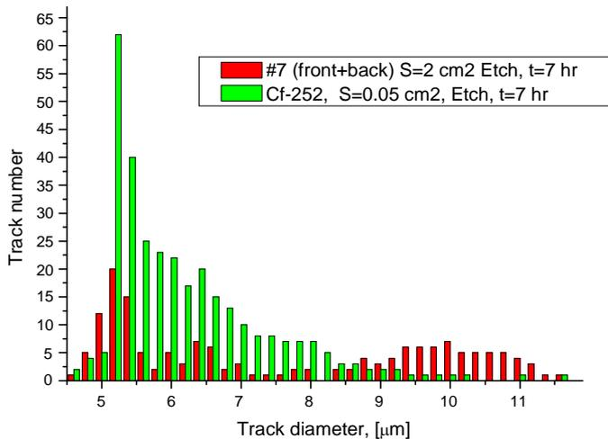
**Figure 7.** Comparison of CR-39 Cf-252 proton recoil spectrum corresponding to 7 hr etching with the sum of spectra obtained from both sides of #7 CR-39. In the track diameter range of 4.5-8.0  $\mu\text{m}$  the #7 spectrum look similarly to Cf-252 recoil. Note, that the maximum of track diameter distribution for the #7 detector is localized near the 5.2  $\mu\text{m}$  value.
