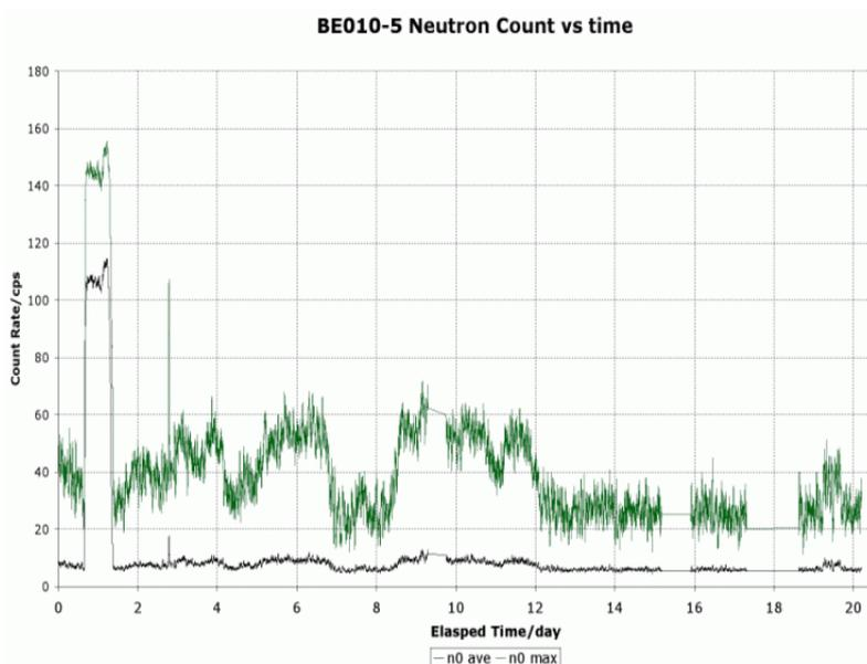
**Figure 20.** Neutron protocols of the run #5 obtained in SRI with the BF<sub>3</sub> detector.
