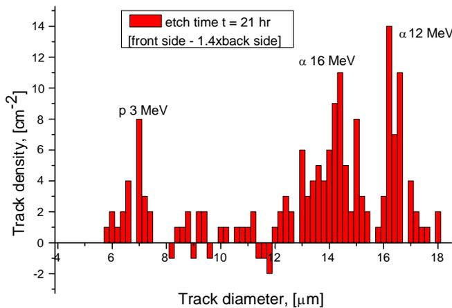
**Figure 19.** The front side spectrum of nuclear tracks of #5 detector subtracting the neutron induced proton recoil spectrum from its back side, at  $t = 21$  hr etch.
