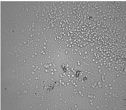
**Figure 13.** Typical image of the front side of the #5 detector at etch time  $t = 7$  hr.
