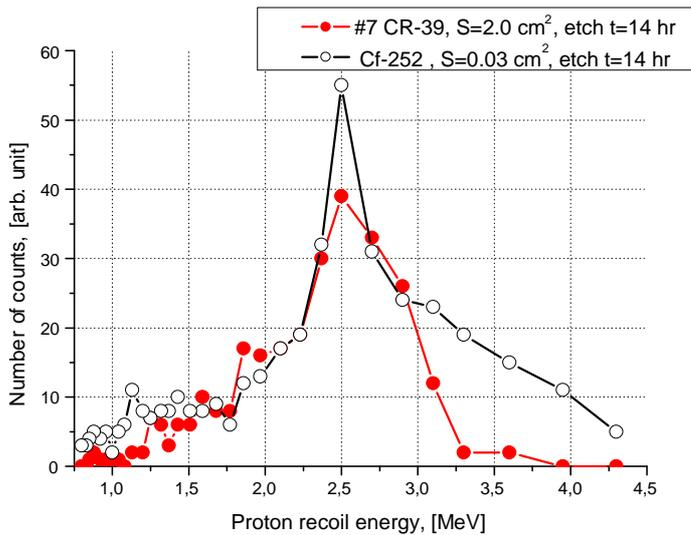
**Figure 12a.** Rough reconstruction of the protons recoil spectra for CR-39 Landauer detectors obtained during electrolysis run (detector #7) and during exposure with Cf-252 neutron source. Etch time is  $t = 14$  hr. The reconstruction of the spectra was deduced from the track density vs. track diameter histograms, taking into account two functions: (a) track diameter vs. proton energies at  $t = 14$  hr, and (b) the critical angle  $\theta_c$  vs. proton energy.
