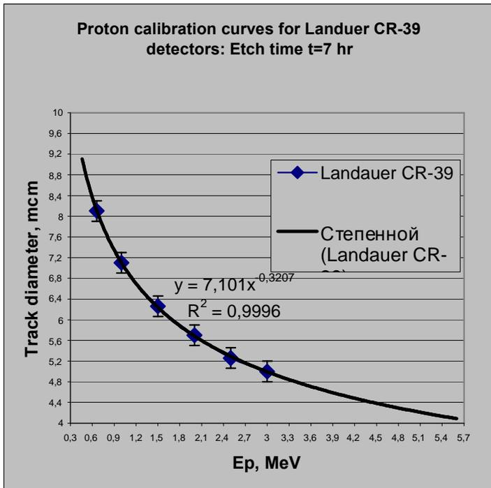
**Figure 3a.** Van de Graaf accelerator calibration curve for the 0.65-3.0 MeV proton beam of normal incidence with respect to the detector surface. The targets are Landauer RadTrack and another Fukuvi-type CR-39 detector. Etching conditions: 6 N NaOH, T = 70°C, t = 7 hr.
