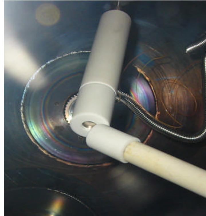
Detector Arrangement – AXUV detector, film and TLD foils – key point – detectors face cathode where D bombardment occurs, not anode with electron bombardment, i.e. x-rays not simple electron Bremsstrahlung
