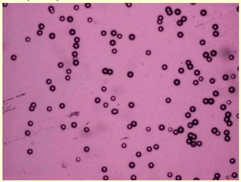
Dorschel et al. 2001 Track diameter, *d*, as a function of the alpha energy, *W*. Etching conditions: 7.25 N NaOH, 70 °C, 6 h.
