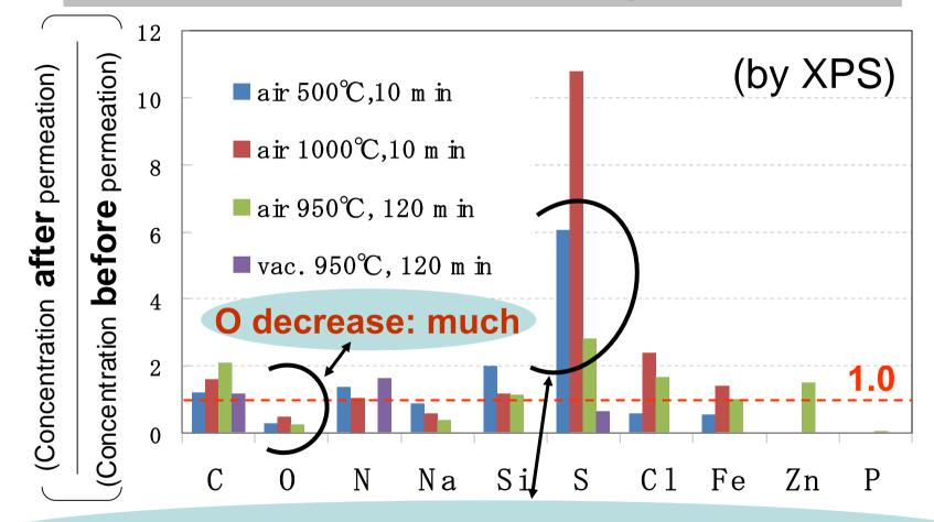
Increase of S is remarkable for the air- annealed samples
