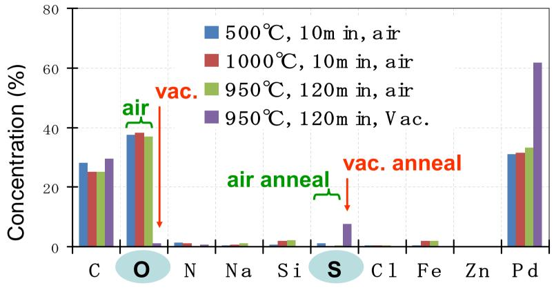
Vac anneal  $\Rightarrow$  high S concentration at the surface Air anneal  $\Rightarrow$  low S concentration  $\Rightarrow$ initial high permeability
