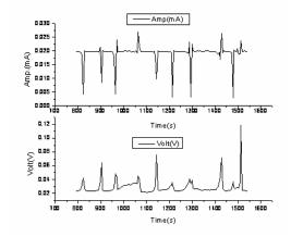
Figure 1. Electrolysis current and voltage pulses by computer multichannel registrated system
