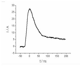
Figure 2. The pulsed current waveform of plasma electrolysis with  $K_2CO_3$  electrolyte
