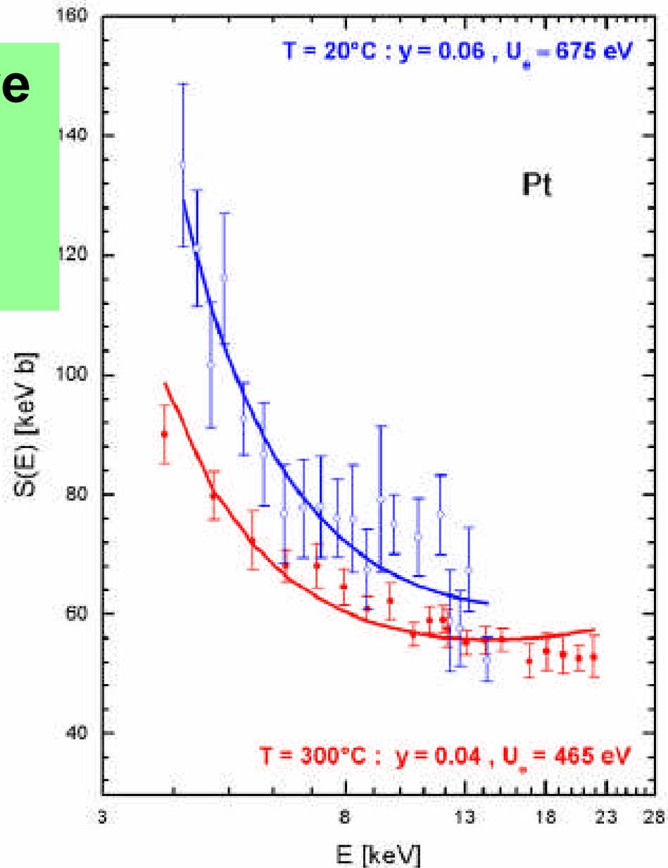
**Figure 1.** The  $S(E)$  factor of  $d(d, p)t$  for Pt at  $T = 20^\circ\text{C}$  and  $300^\circ\text{C}$ , with the deduced solubilities  $y$ . The curves through the data points include the bare  $S(E)$  factor and the electron screening with the given  $U_e$  values.
