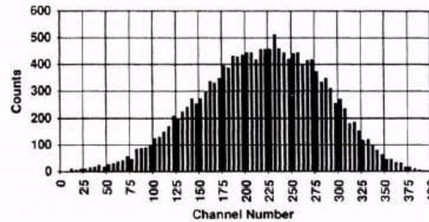
Fig. 3 Beta spectrum of secondary tritium standard: Tritiated H<sub>2</sub>O (1000 dpm) in Beckman scintillation cocktail. Ordinate: Counts per 5 channels per minute.
