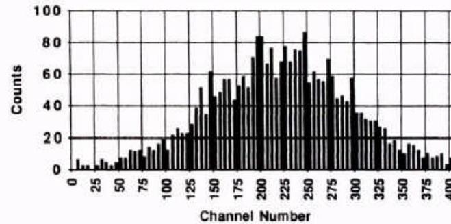
Fig. 2. Beta spectrum of Pd cathode piece after D<sub>2</sub>O electrolysis and application of closed-system analytical method.<sup>6</sup> Ordinate: Incremental counts per 5-channel interval in 20 minutes.
