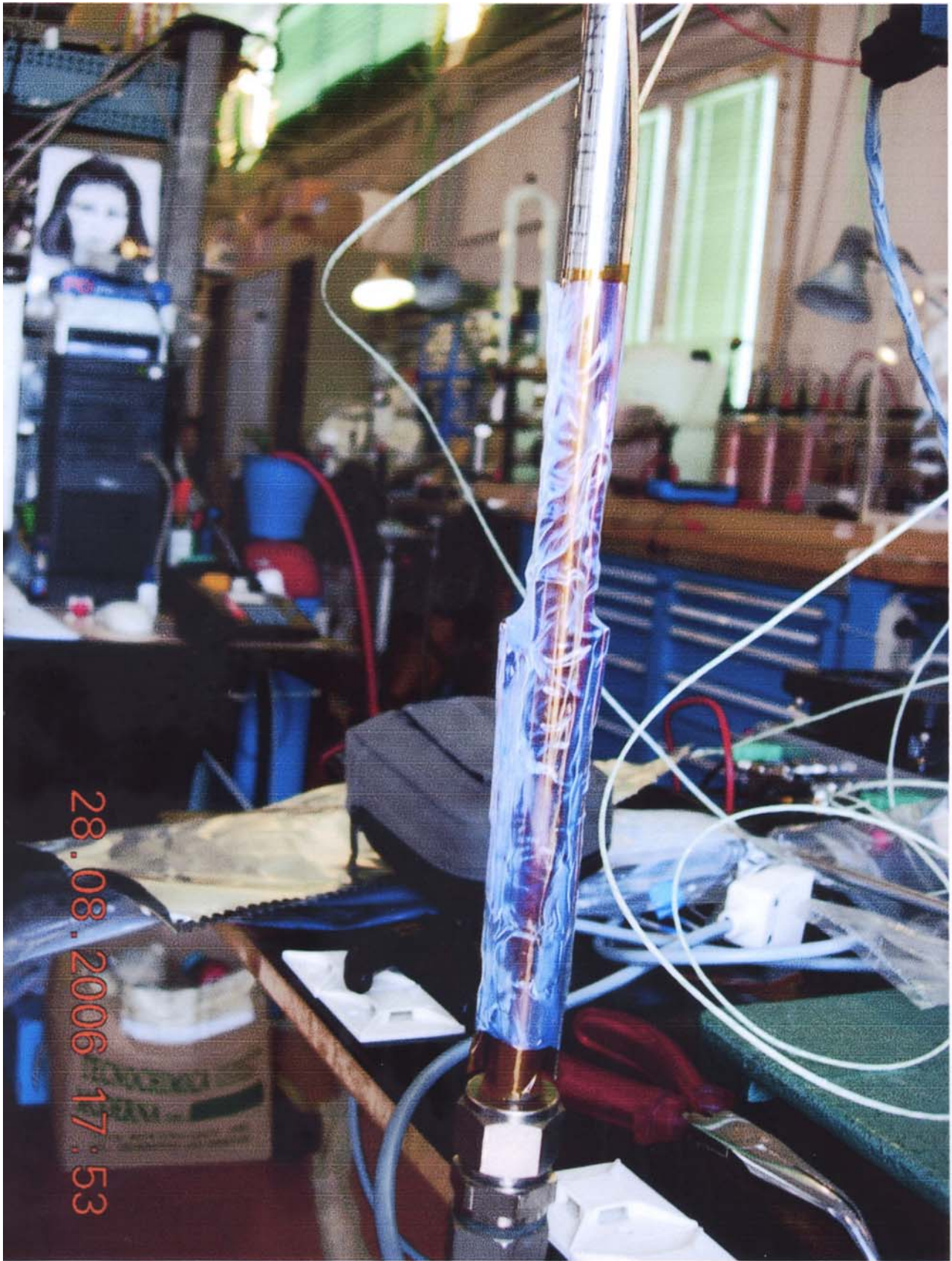
Fig. 19 Detail of the multilayer reaction chamber V2 during assembling.
