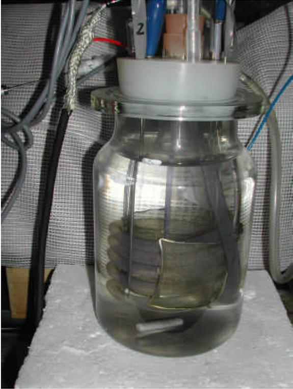
**Figure 1. A glow discharge cell. Photo taken in 2003 by T. Mizuno**
